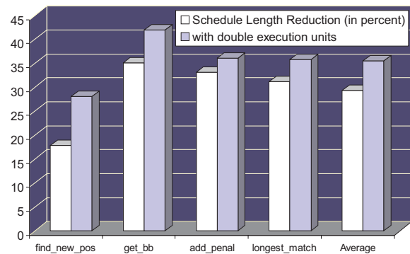
Figure 8: Global schedule length improvements over Intel’s compiler on the same Itanium 2 target processor (left bars) and on a processor with the double number of execution units (right bars).
